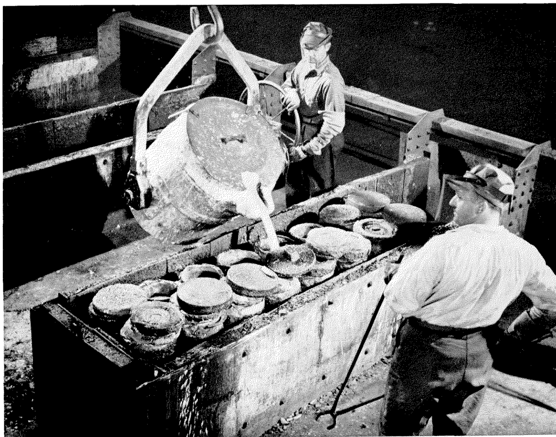
Basic to the Copperweld process is the pouring of molten copper around a heated alloy steel billet centered in a mold. The resulting ingot is reduced by hot rolling and cold drawing to final wire size.
